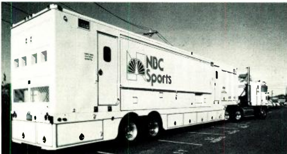
AF Associates built the N-1 mobile unit for NBC Sports. Audio section is fully stereo-capable.
