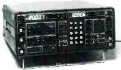
The Model 5500 from Amber runs through distortion and noise tests automatically.
