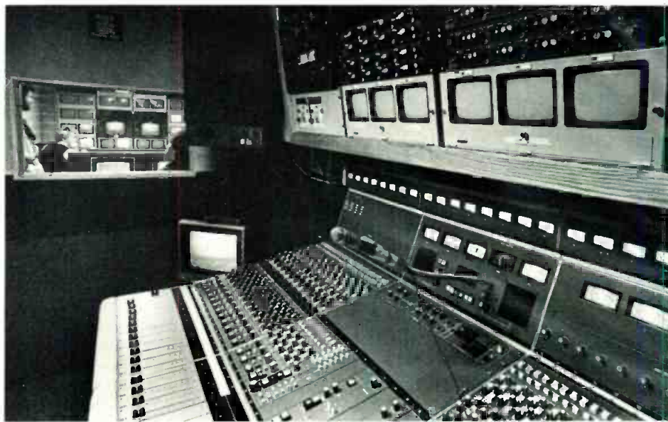
Reeve's Teletape's largest truck, used for Live from Lincoln Center, carries a Neve 5114 console.
