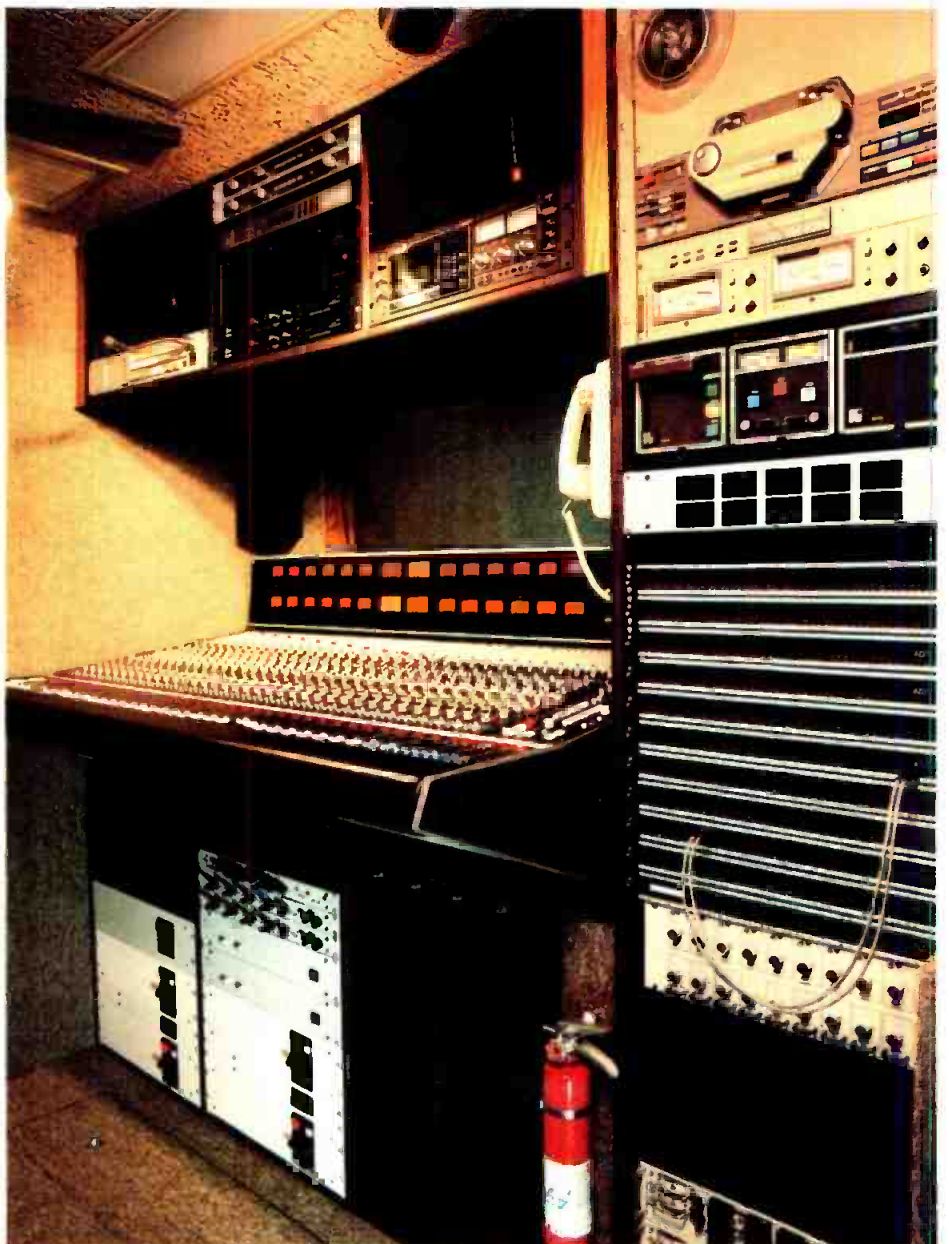
Audio area of Centro-built KWGN-TV truck has a Neotek audio board, Tascam reel-to-reel ATR, and ITC cart decks.
