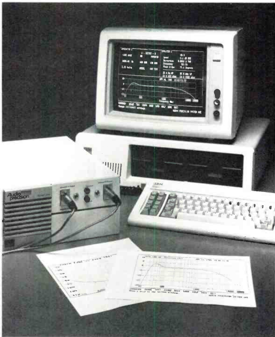
Audio Precision's System One selects entire test procedures or changes instrument settings via an IBM PC.
