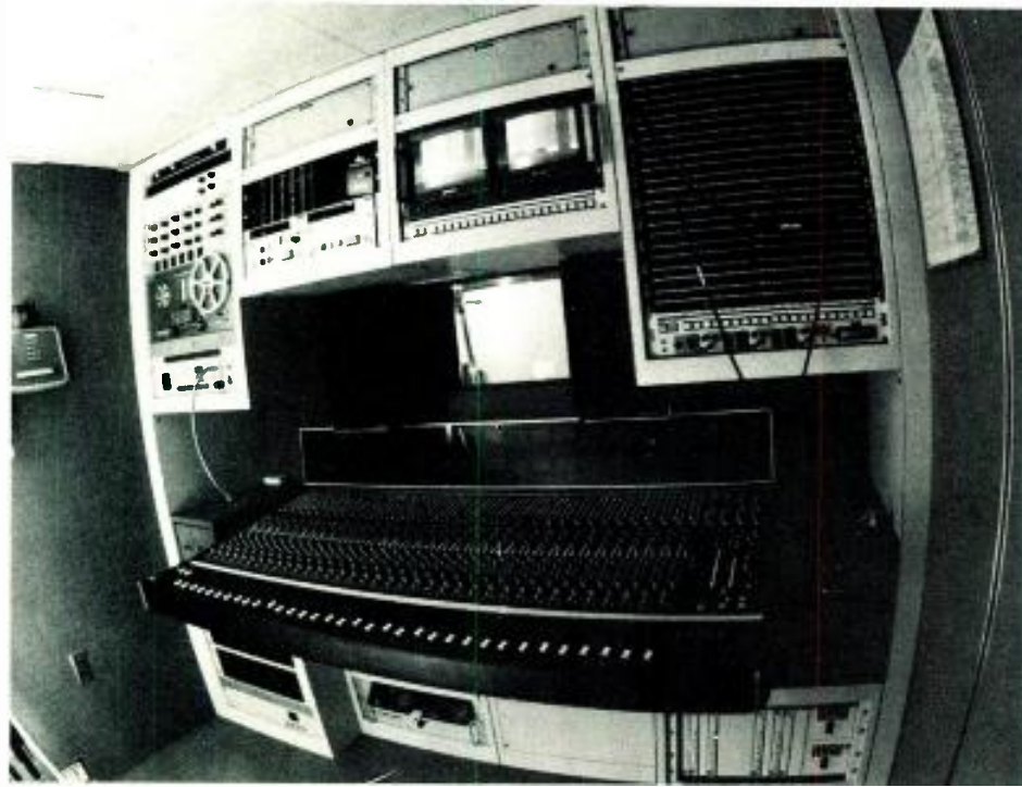
Auditronics console with 36 inputs gives CRT's Roscor-built truck the audio muscle it needs for stereo jobs.
