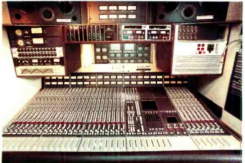
Built by Midwest Corp. with stereo in mind, Turner Broadcasting's new truck has an automated SSL audio console.
